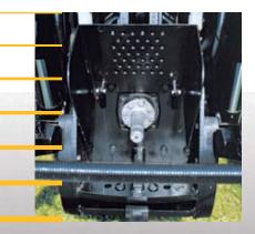
The MT565 and MT635 are equipped with a PTO that operates at both 540 and 1,000 rpm, and PTOs on the MT645, MT655, MT665 operate at 1,000 rpm.
