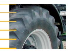
The Agribib tubeless radial tire is designed to deliver all of your tractor's power to the ground, with minimum slip and maximum traction.
