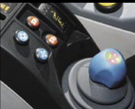
The joystick lets you easily and precisely program function and flow settings, record them in the TouchMaster memory and repeat them with a single move of the joystick.
