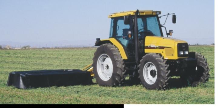
Challenger three-point hitch-mounted disc mowers are built with field-proven cutterbar technology. Whatever you're cutting, alfalfa, fescue, Bermuda or orchard grass, these mowers are designed to deliver years of quick, clean cuts and dependable service under the toughest field conditions.
