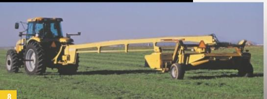
The conditioner rolls are mounted to the header rather than to the frame, so the crop feeds uniformly into the conditioner rolls. The rolls are wide enough for the crop to spread out evenly for uniform crimping.
