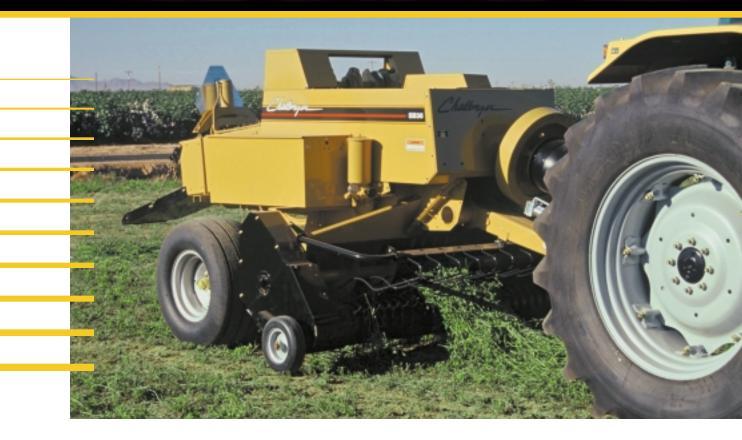
Challenger centerline balers are technologically advanced, fast and rugged with the features you want and need to produce high quality bales. They produce popular-sized bales that are easy to handle, small enough to be stacked and fed by hand, and solid enough for long-distance hauling and storage.
