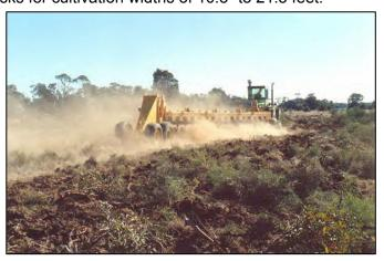
The deep cutting action of individual jump arms and disks **effectively penetrate and kill the root system of Mesquite** brush that reduces grass production for grazing
