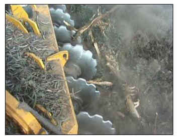
Patented Stump Jump hydraulic arms and disks provide adequate depth of penetration in any soil with relief over rocks and stumps with minimal maintenance.
