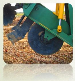
The abrasion resistant steel coulter mounted in front of the sub-tine eliminates chocking with roots and reduces pull force by 25%. The Savannah original ripper has hard changeable insert to ensure longer durability and easier maintenance
