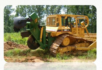
The Magnum 420 Mounted Sub-Soil Plow provides a high tilled 1.5m wide bed with an adjustable ripper designed for shallow 100% tillage or deep compacted soil sub-soiling. The disc configuration permits a better cutting action in debris and provides finer tillage, which assists in improved moisture and mineral retention, as well as herbaceous control. Runs on 180hp or greater dozers. "N" Model is a narrow version that cultivates 1.2m wide.
