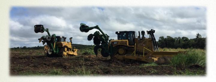
The Magnum 430N Mounted Sub-soil Plow has a "No Profile" tillage configuration. Discs are set with less pitch, allowing closer spacing, less drag, and greater cutting action. With less aggressive discs, fine tillage is achieved and provides a dense soil structure free of dirt clods and air pockets without an additional packer or chopper roller. The Magnum 430N has 1.6m working width.
