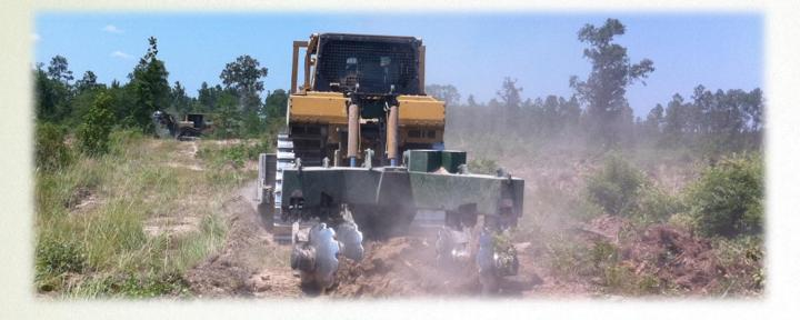
The Magnum 440 Mounted Sub-soil Plow provides a 2.3m wide well-defined bed over the rip-line. Runs on 250hp or greater dozers and, same as all the other Magnum 400 Plows, has mounts to add a packer or chopper roller to improve the compaction and density of heavy soils.
