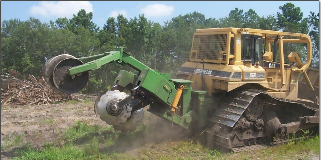
Savannah® Magnum 240 with Radial Lift Assembly mounted to Caterpillar D6R
