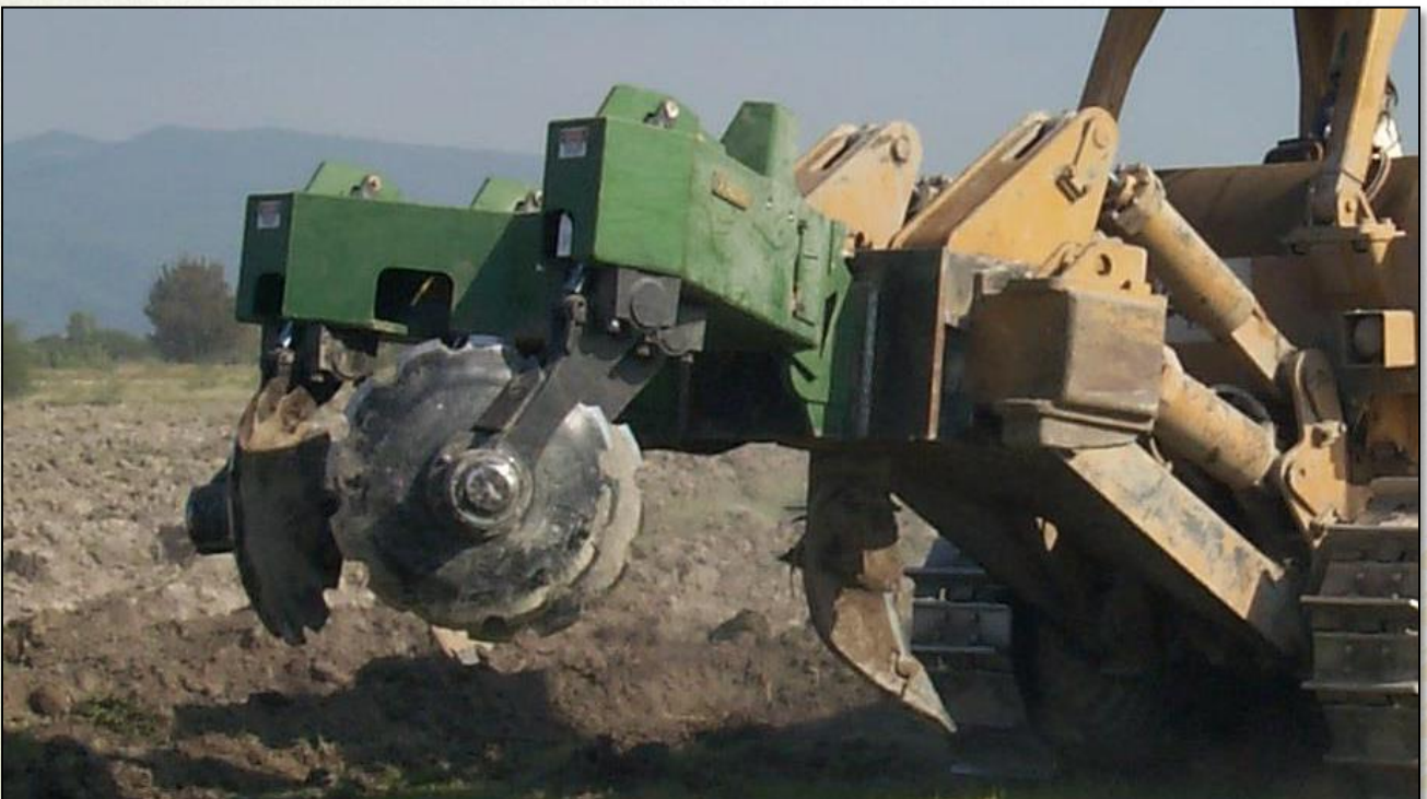
Savannah® Magnum 240 with J-Hook Quick Release Ripper Mounts mounted to a CAT D8K
